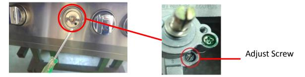
3. Use flat head screwdriver to rotate about 45 degrees clockwise. The flame will be turndown.
