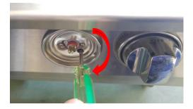
4. Test one burner at one time, and check if the flame is stable. (If low heat flameout or unstable situation happen, please rotate to counter clockwise with a flat head screwdriver until the fire will not flameout.)
